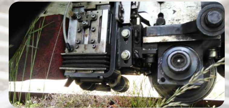
ET System for Headchecks Detection on Rail
