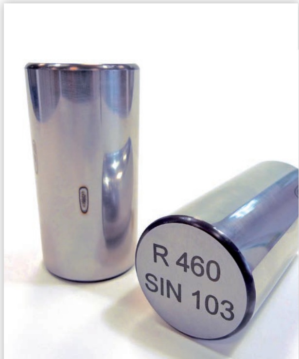
ibg crack and grinder burn master with EDM cracks and pores for simulation of surface open defects and with laser defects for simulation of grinder burn; intensity mere residual stress (cutting far left) and beginning annealing zone (left).
