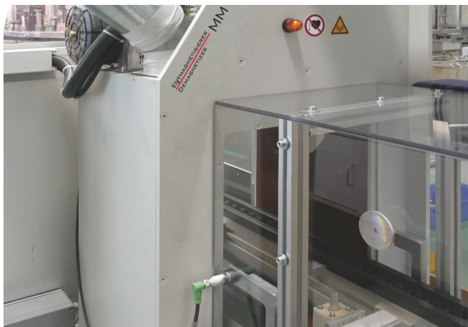
VE with integrated light barrier for pulse triggering. This allows the system to work autonomously
